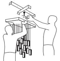
**8.** Once the canopy is installed, untie the wires, gently stretch them down - go few times on each wire. Insert the bulbs and check they all work.
