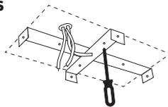
**6.** Connect the positive wire from your electrical box with the positive labeled wire of the Lighting Fixture, Use the twist connector attached to the positive wire of the Lighting Fixture in order to connect between these 2 wires.
