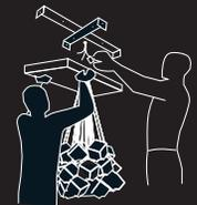
**6. Once the canopy is installed, untie the wires, gently stretch them down - go few times on each wire.**
